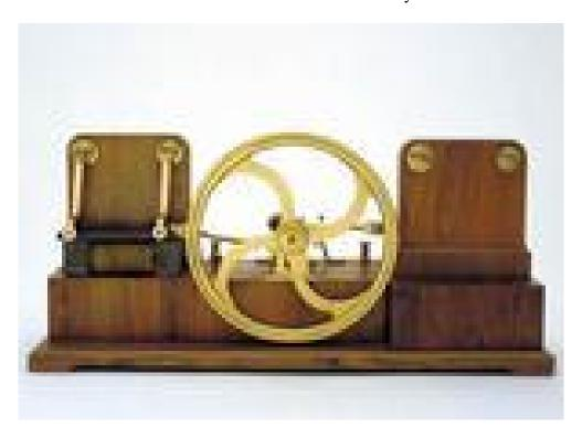
Electric motor probably made for the physicist Luigi Magrini. It is mounted on a wooden block attached to the base. The large brass wheel is rotated by a double crank, also linked to the commutator. Two electromagnets are energized in turn, each one attracting a steel plate (armature) suspended by two rocking arms hinged to a wooden upright. A brass rod connects the system to one of the two cranks. The motion thus resembles that of steam-engine pistons. Provenance: Lorraine collections
